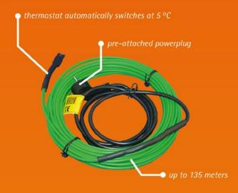
The system is easy to install, you fix the heating cable with tape on the pipe and the plug will ensure a quick installation. Depending on the pipe diameter and thickness of insulation you have a frost protection against -20 °C or -30 °C. We refer to the technical installation manual for an exact overview of your desired pipe diameter and insulation.
