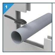
Make sure that the service penetration and the gap are free from dust, dirt and grease.
