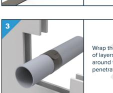
Wrap the required number of layers of Multiwrap around the service penetration.
