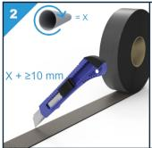
Measure the circumference of the service penetration and cut the Multiwrap to size with a knife. Remember to keep an extra length of at least 10 mm to create an overlap.
