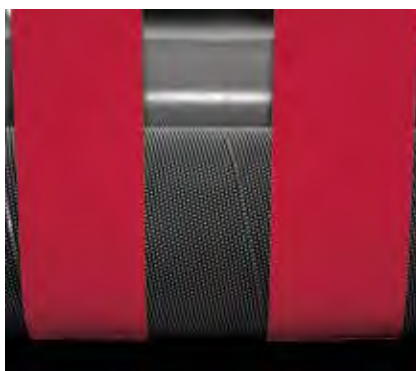
Sample: Coroplast 812 X (black/anthracite tape) used to cover roller when winding on adhesive tape (red tape)
