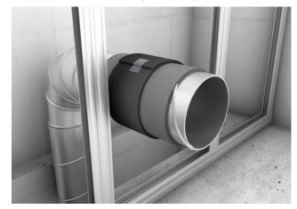
The annular gap is sealed with a gypsum filler (A1) through the whole thickness of the wall.
