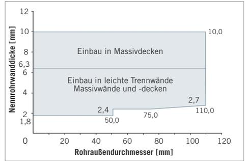
Diagramm 2: Rohre aus PE-HD, PE-LD, PP, ABS, ASA, PE-X, PB, PS
