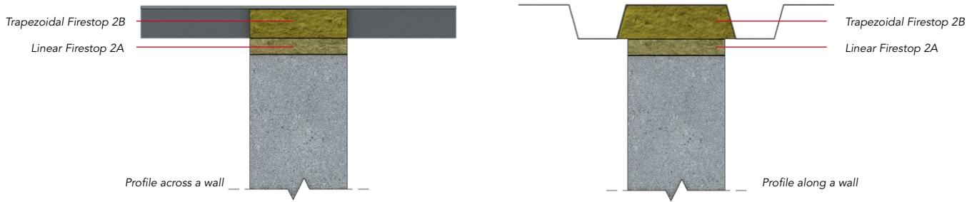
Figure 4 Profiled metal deck over blockwork wall
