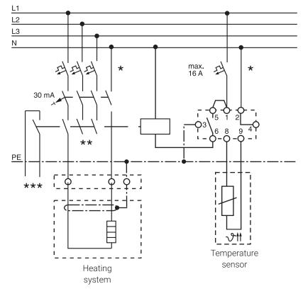
\* Two- or four-pole electrical protection by circuit-breaker may be needed for local circumstances, standards and regulations
