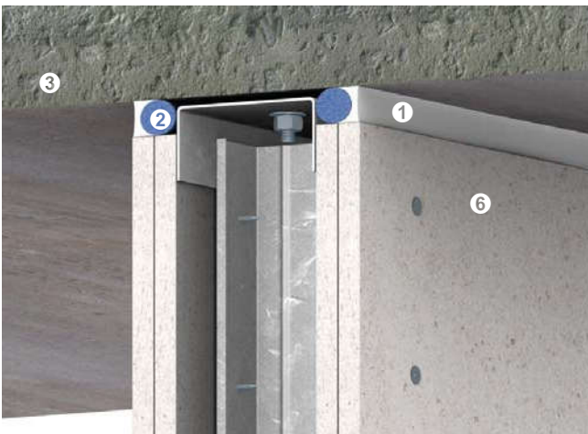
Typical head joints of lightweight partition (STC 45-50)
