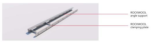
For fixing to timber, the ROCKWOOL clamping plate is used, compressing the barrier to the timber, fixed at 450mm centres using No. 10 woodscrews.
