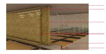
Concrete soffit 2mm tested angle fixed to soffit at max 750mm
