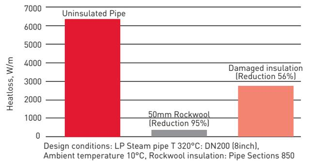
Between 10% to 30% of the insulation becomes damaged or missing within 1 to 3 years
