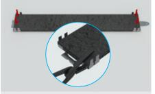
4. Place the strip on a surface. The intumescent part has to be visible. Fix the closing bracket A on one end of the strip and B on the other end e.g. by using tongs (when you hear a clicking sound, then the brackets are correctly attached);
