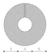
CLIMAFLEX® XT has approved self-adhesive strips, which reduce the processing time of previously installed pipes by up to 50%. Simply peel off the protective film, press down and it's done.
