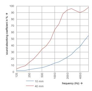
Absorption material : SonoBaffle FL CIL, cilinder
