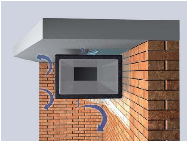
Figure 3: Build-up zones prevent convective heat transfer
