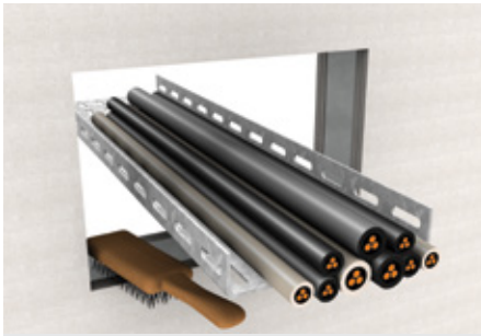
1. Clean aperture opening and penetrating services
