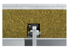
At duct flanges, the slabs need to be cut to fit. The same principle applies for slab joints as well as for slab passages (see picture opposite).
