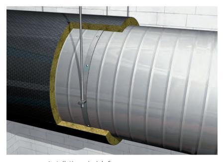
Installation principle for horizontal circular ducts
