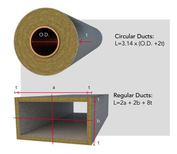
Thickness of ROCKWOOL insulation for chilled air ducts (taken from BS 5422:2009 Table 12)
