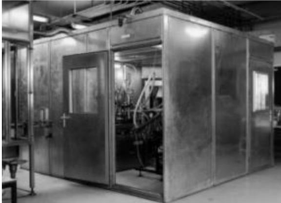
**Product description** The Sonodamp tailor-made sound-insulating and sound-absorbing enclosure are available in steel, stainless steel or aluminium
