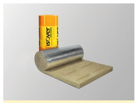
U Protect Roll Alu1 provides topclass thermal insulation for hot water and heating pipes and secures the building fire safety for penetrations up to El 120 according to EN 1366-3. Rolls are easy to wrap around big diameter pipes and pipe clusters. Alufacing provides efficient water vapour barrier when intact and seems carefully taped.
