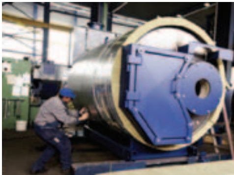
Insulation works on a fire tube boiler with ProRox MA 520 ALU
