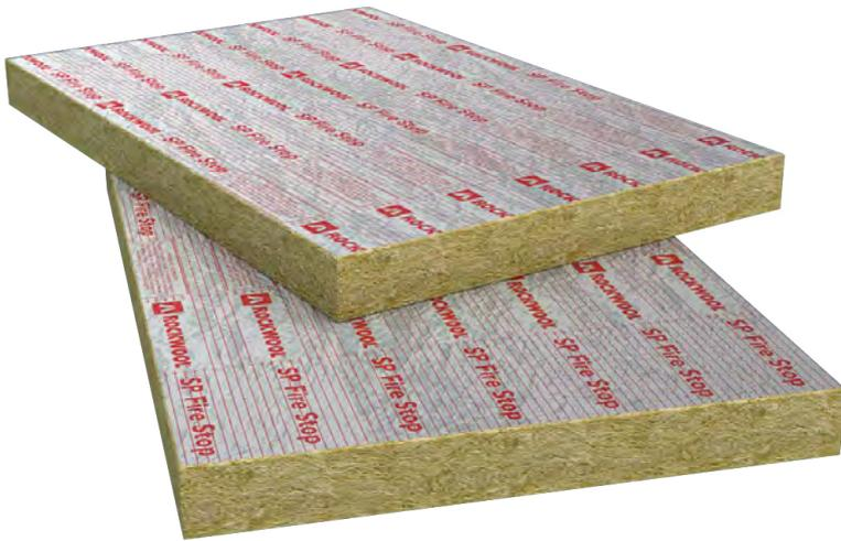
The ROCKWOOL SP FireStop System comprises of both the SP FireStop Slab, SP FireStop Plus Slab and SP FireStop fixing brackets. SP Slabs incorporate a foil facing to both sides which helpfully includes cutting lines to support accurate installation.
