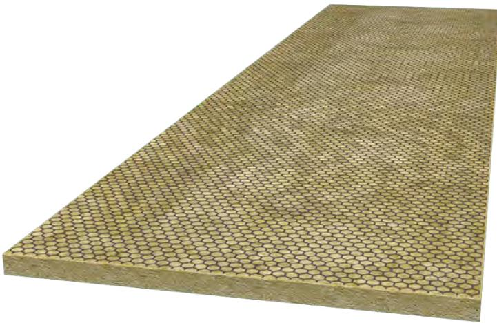
ROCKWOOL Fire Barrier is comprised of stone wool and has a galvanised wire mesh which is stitched to one side. Foil faced options and double sided wire mesh are also available. Fire Barrier systems have been developed to prevent the spread of flames and inhibit heat and smoke through concealed spaces in buildings and improve sound reduction.
