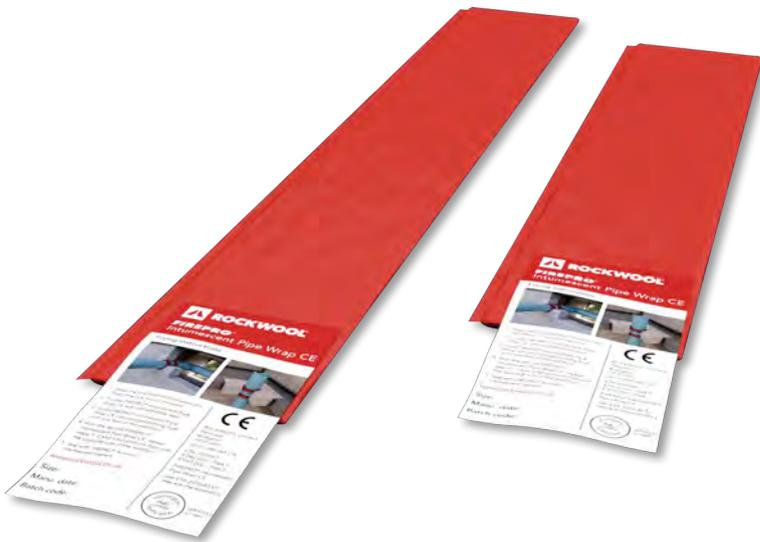
Intumescent Pipe Wraps CE are designed to seal service penetrations in apertures containing combustible plastic pipes. Pipe Wraps CE comprise layers of a graphite based intumescent sheet encapsulated in a polythene sheath. All Pipe Wraps CE are supplied in correct lengths to suit the pipe diameter.
