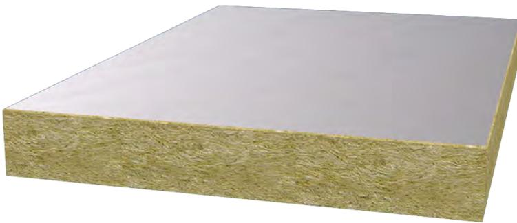
ROCKWOOL Fire Barrier Slab comprises a high density stone wool core which is foil-faced on both sides. Fire Barrier Slab has been developed to prevent the spread of flames, inhibit heat and smoke through concealed spaces in buildings and improve sound reduction.
