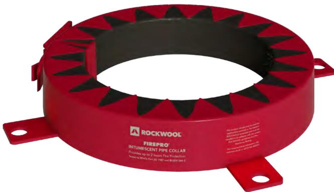
Tested to the harmonised European Standard EN 1366-3:2009, FIREPRO® Pipe Collar CE provides up to 4 hours\* fire stopping in rigid floor constructions and up to 2 hours fire stopping in flexible/rigid wall constructions.
