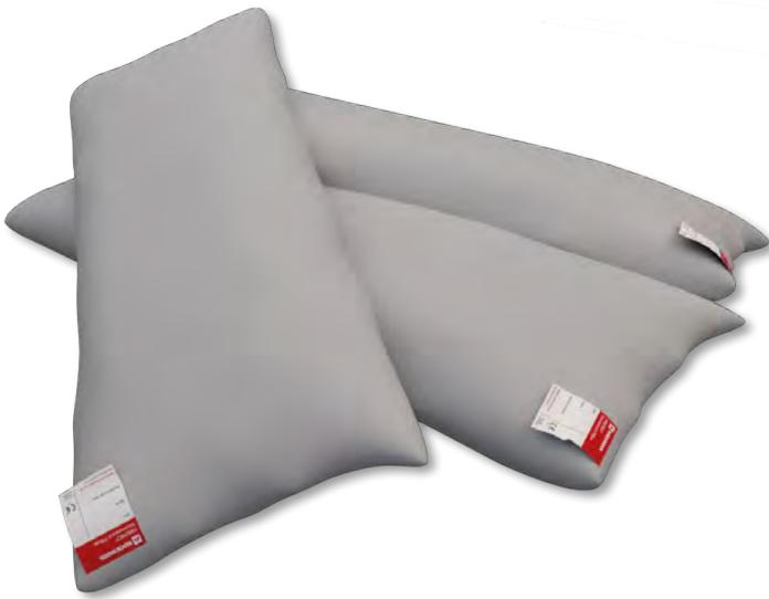
FIREPRO® Intumescent Pillows CE consist of intumescent material encased within a waterproof glass cloth bag. Intumescent Pillows CE are designed to create a temporary or permanent fire seal around all types of services to maintain continuity of fire performance of compartment walls. They are an ideal solution for applications where services are required to be changed or replaced on a regular basis.
