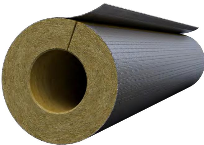
RockLap H&V Sections are pre-formed sections of stone wool insulation. Manufactured pre-slit and provided with a factory applied foil facing complete with integral self-adhesive lap.
