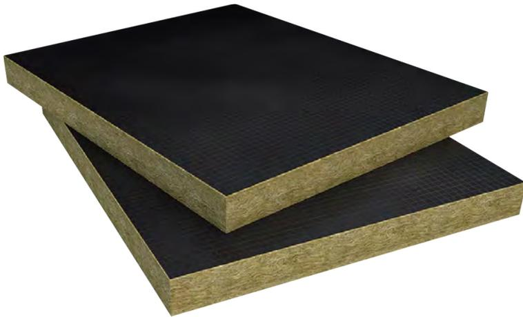
**Tested to both BS EN 1366:Part 1 and BS EN 1366:Part 8 FIREPRO® DuctRock® Slab is capable of providing up to 2 hours fire resistance to rectangular ventilation and smoke extract ductwork.**
