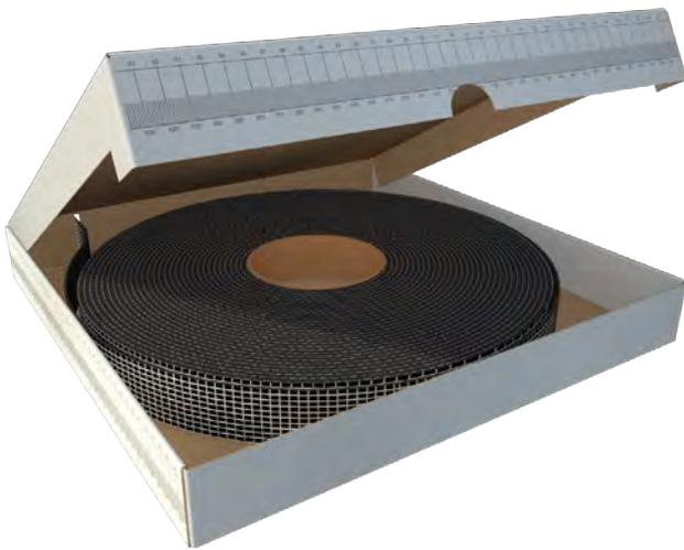
Intumescent Pipewrap Roll comprises an intumescent material made from elastomeric thermoplastic polymers combined with active components that provide a high volume expansion and pressure seal in the event of a fire.
