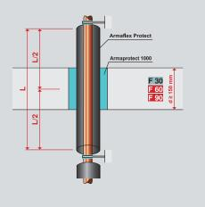
Armaflex Protect can also be installed centrally in ceiling penetrations. Armaprotect 1000 or mineral mortar is used to close the remaining gap in the penetration or core-drilled hole.
