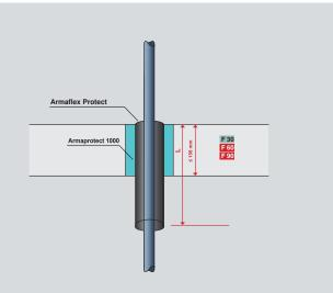
Under-ceiling insulation in the case of plastic pipes.
