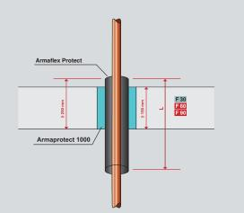
If no insulation is required or possible above the ceiling, Armaflex Protect can be installed under the ceiling. In this way radiator connections, for example, can be sealed off simply and safely.
