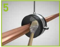
Wet seal the butt joints using Armaflex adhesive.
