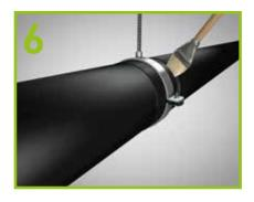
Install Armaflex insulation on either side of the pipe support. Ensure that the pipe insulation is installed under slight compression.
