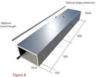
Rectangular ducts - 45° mitre joint system, showing installation sequence
