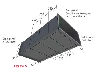
Steel pin arrangement where side panel does not exceed 1000mm and soffit panel does not exceed 600mm
