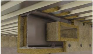
Figure 10 Beam with square or rectangular holes (boxed protection - dry joints)
