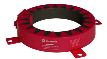
Tested to the harmonised European Standard EN 1366-3:2009, FIREPRO® Pipe Collar CE provides up to 4 hours<sup>\*</sup> fire stopping in rigid floor constructions and up to 2 hours fire stopping in flexible/rigid wall constructions. \*Subject to the application
