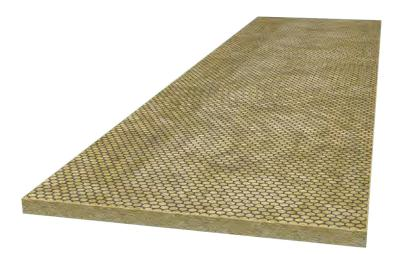
ROCKWOOL Fire Barrier is comprised of stone wool and has a galvanised wire mesh which is stitched to one side. Foil faced options and double sided wire mesh are also available. Fire Barrier systems have been developed to prevent the spread of flames and inhibit heat and smoke through concealed spaces in buildings and improve sound reduction. Approved for LUL applications
