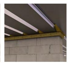
Figure 3 Linear Firestop 2A and Dovetail Infill Strip
