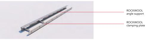
For fixing to timber, the ROCKWOOL clamping plate is used, compressing the barrier to the timber, fixed at 450mm centres using No. 10 woodscrews.
