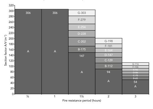
The following key provides the required minimum thicknesses of ROCKWOOL BEAMCLAD® for the Section Factors given in the tables above.
