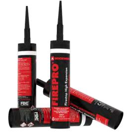
ROCKWOOL FIREPRO<sup>®</sup> High Expansion Intumescent Sealant is water based acrylic sealant containing graphite. In the event of a fire, the active components provide a high volume expansion and pressure seal, closing off the void left by combustible materials.
