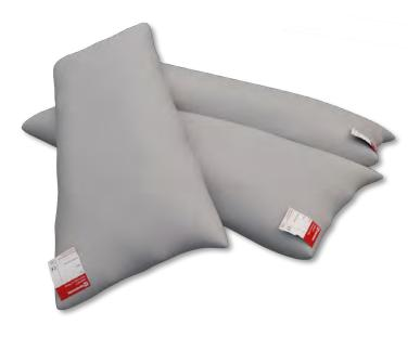
FIREPRO® Intumescent Pillows CE consist of intumescent material encased within a waterproof glass cloth bag. Intumescent Pillows CE are designed to create a temporary or permanent fire seal around all types of services to maintain continuity of fire performance of compartment walls. They are an ideal solution for applications where services are required to be changed or replaced on a regular basis.
