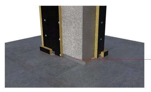
40 x 40 x 3mm galvanised steel L-profile fixed with 3.2 x 15mm self tapping screws to the duct and 7.5 x 62mm screws to the floor.
