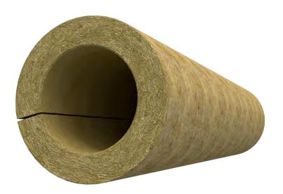
FIREPRO Fire Tube is a pre-formed cylindrical insulation manufactured using ROCKWOOL stone wool. The product is available with an optional aluminium foil facing.
