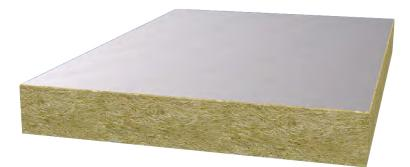
ROCKWOOL Fire Barrier Slab comprises a high density stone wool core which is foil-faced on both sides. Fire Barrier Slab has been developed to prevent the spread of flames, inhibit heat and smoke through concealed spaces in buildings and improve sound reduction.
