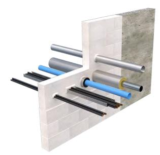
HS Firestop Compound is a specially formulated gypsumbased mortar, which is mixed with water to create a workable range from stiff to pourable mix. HS Firestop Compound is also suitable for pre-casting into convenient size blocks for use in wall openings.
