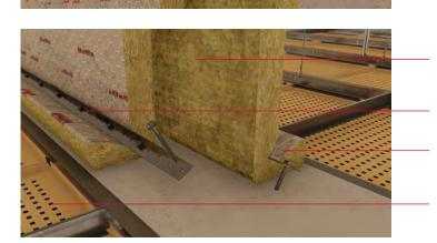
Two layers of foilfaced Fire Barrier
