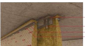
2mm tested angle fixed to soffit at max 750mm centres
