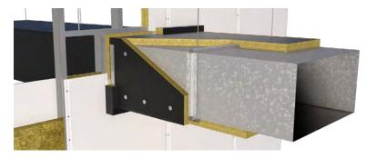
Figure 8 ROCKWOOL Patented Dry Wall Penetration Detail
