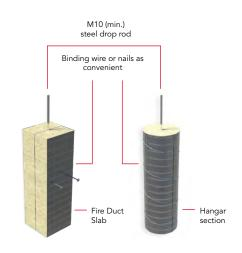
Figure 5 Isometric view of drop rod protection options
