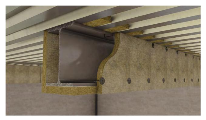
Figure 1 Stud welded pin, dry joint board system
