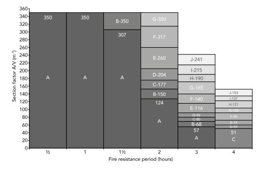
Chart 3 - Steel beam sections ROCKWOOL BEAMCLAD® glued joint systems: Critical steel temperature 620°C
