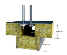
Figure 4 Protection using block cover strip
