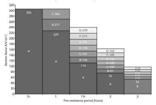
Chart 1 - ROCKWOOL BEAMCLAD<sup>®</sup> stud welded pin dry joint system: Critical steel temperature 620°C, 3 sided protection for beams
