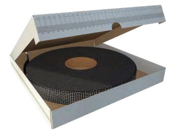
Intumescent Pipewrap Roll comprises an intumescent material made from elastomeric thermoplastic polymers combined with active components that provide a high volume expansion and pressure seal in the event of a fire.
