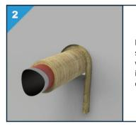
If backing is applied, cut it slightly wider than the gap width and make sure that it is applied to the correct depth in the structure.
