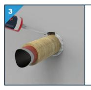
Apply Multimastic SP generously in the gap to prevent air bubbles.
