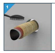
Make sure that the service penetration and the gap are free from dust, dirt and grease. Moisten the structure, if necessary.
