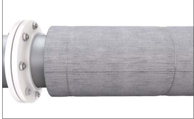
Figure 20: Termination next to a flange: bolt clearance
