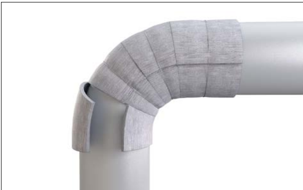
Figure 36: Securement of segments using insulation wire.
