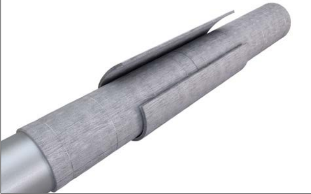
Figure 13: Staggering of next layer of ArmaGel.
